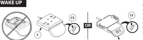
NOTE: For Programmable Paddles (C) only. Paddle (C) enters a power save mode after 10 seconds of inactivity. Prior to each use, user must "TAP AND RELEASE" paddle (C) or "TAP AND RELEASE" the menu button (C3) to activate paddle (C).
