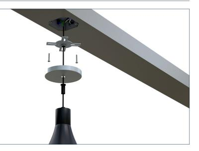
• Lighting attached to underside of Light Trough • Maximum of two prep locations per Light Trough • Center, one-side, or outside (x2) prep options available • Max Weight of Light (1 box) – 50 lbs (22.7 kg) • Max Weight of Lights (2 boxes) - 100 lbs (45.5 kg) evenly distributed between two boxes
